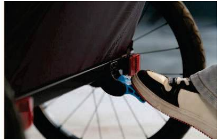
The parking brake can be fixed by placing the foot on the foot brake.
